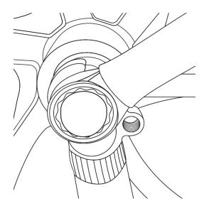
Attach the pedals to the bike by using a 15mm wrench, be sure to identify the correct pedal for the correct side, there is a R or L marked on the end of the pedal bolt. Be sure to note that the left pedal is reverse threaded. It is recommended to add general purpose grease to the threads before installing the pedals. (Right and Left is determined when sitting on the bike)
