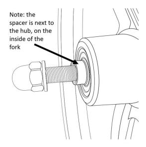
The Right side of the wheel will use the wider 8.5mm spacer between the hub and fork as shown below.
