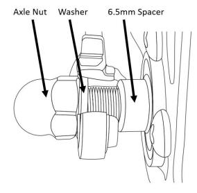
Then use a 16mm wrench to tighten the axle nuts firmly. As shown below.
