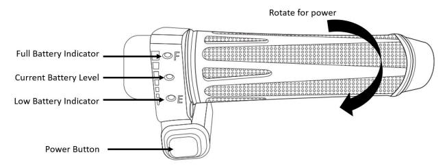
First, press the power button to turn on the bikes electrical system, the battery indicator will light up showing the bike is now powered on.
