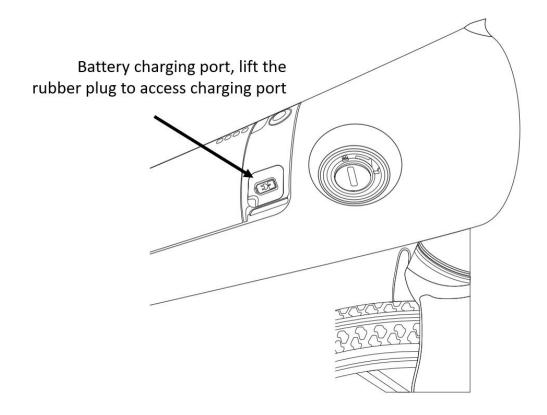
Install the charging plug into the battery charging port, as shown below.
