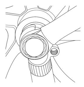
Flip the bike over onto the wheels and be sure to check that the handlebars are aligned with the front tire. Then tighten both sides of the stem to the fork using a 4mm Allen wrench, tighten to 45 IN-LBS or 5 Nm.
