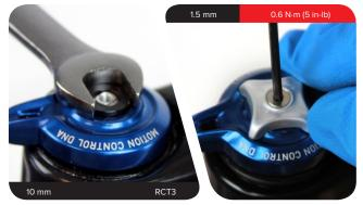
$\ensuremath{\textbf{RL:}}$  Install the lockout adjuster knob on the top cap so the knob rotates from open to closed.
