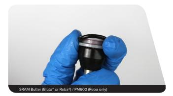
Remove the top out bumper cone from the air piston. Inspect the tension pin hole on the air piston. Install the top out bumper cone onto the air piston.
