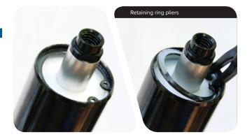
Remove the rebound damper and seal head.
