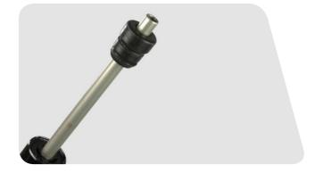
Push the air shaft into the upper tube to prevent it from getting scratched while removing the retaining ring.
