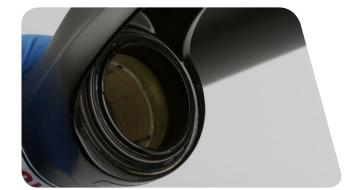
Stabilize the lower leg on a bench top. Place the tip of a downhill tire lever under the wiper seal. Press down on the downhill tire lever handle to remove the seal.
