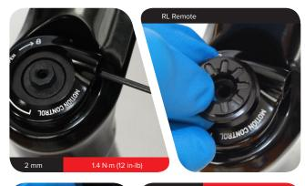
Install the cable spool top so the indicator dot on the cable spool is oriented within the bracket printed on the cable stop. Install and tighten the set screw.
