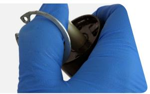
Firmly pull on the air shaft to remove the air spring assembly from the upper tube. Clean and inspect the assembly for damage.
