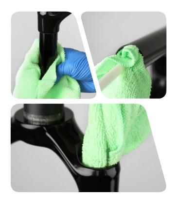
Remove the seal head assembly from the air shaft. Clean the air shaft assembly.
